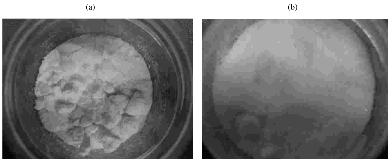
Fig. 1. Pictures of the finished \text{EuD}_4\text{TEA} samples synthesized with (a) europium acetate and (b) europium nitrate. These pictures were taken under standard white room light.
