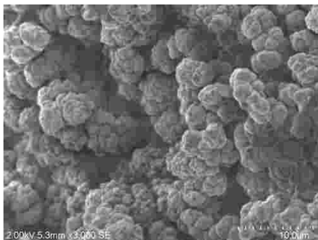
Fig. 12 SEM images of poly(GMA-EDMA)-arginine monolithic column prepared with organic solvent under acidic condition with the optimum condition polymerization.
